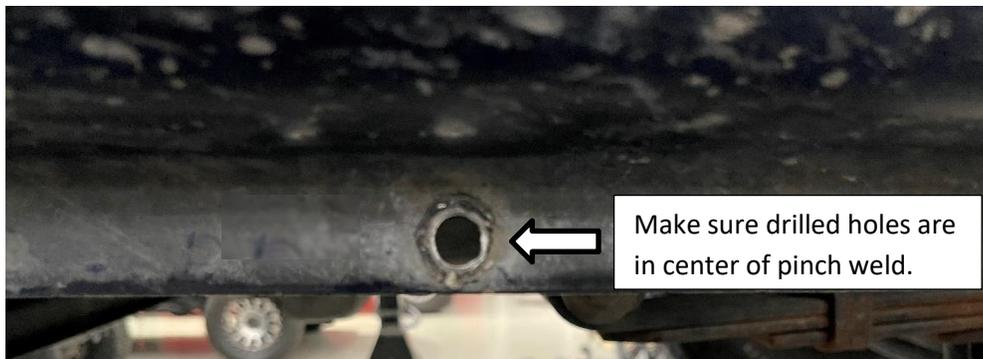
**Step 6.** Align the brackets up with the drilled holes and attach using the supplied 5/16" carriage bolt, nut and washer. **\*\* NOTE\*\*** *The carriage bolt will start from the outside and fasten from the backside of the pinch weld.*
